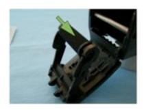
The ink roller is now easily accessible and can be easily replaced by a new one. Please always use genuine parts in order to prevent clogging of the characters and misprints or smearing as a result.
