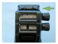
After setting all the characters in the right position for both lines one needs to secure the turning knob in its original position again. In this way the printing is secured.
