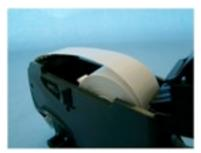
Unroll the label roll partly and take off about 8 labels. Push the roll into the label gun as per picture. The labels are pointing toward the top of the label gun.
